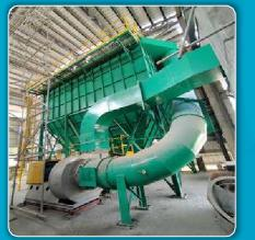
Northern Cement Corporation 8,000 CMH Cement Grinding Dust Collector
