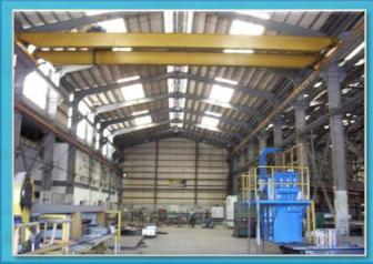
Fabrication Shop -6 bays with 10 tons **Overhead cranes**
