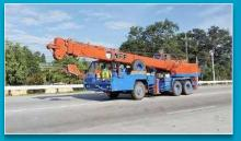
**KATO** 25 tonner Telescopic Truck Mounted Crane
