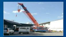
**GROVE** 45 tons Telescopic Truck Mounted Crane
