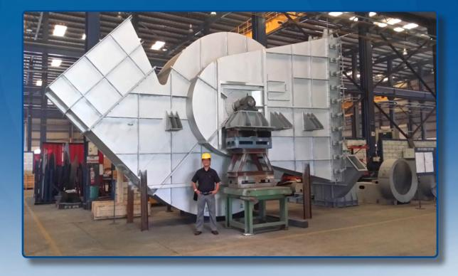
High temperature, dusty, sticky materials are handled by the process fans in the cement plant like Mill Vent Fans, Cooler Vent, Separator Fans and Bag House/EP Fans. Reitz has constantly developed improved designs for high efficiency process fans for the Cement Industry.
